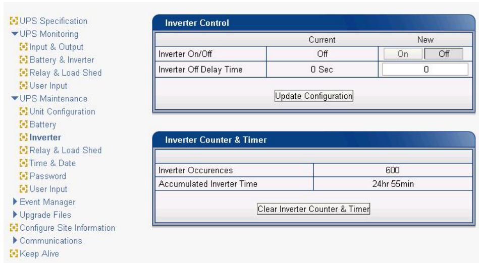
Figure 39 — UPS Maintenance: Inverter screen
